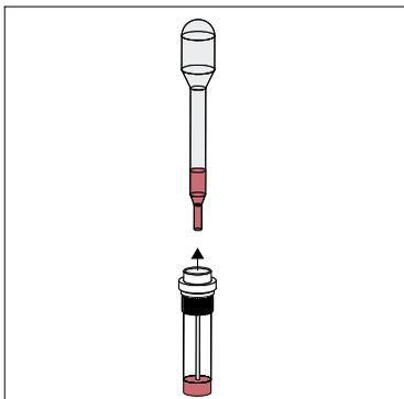
Use the pipette to remove a few drops of the diluted sample.
